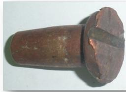
**Fig. 8.** *The nature of wear and damage to the working surface of the contact welding electrode (erosion and crushing of the working surface)*
